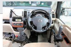
A driving system of a 2-joystick type. It is possible to operate the blinker, horn, brake lock switch, etc. to accompany steering wheel operation in the vicinity of the joystick.
